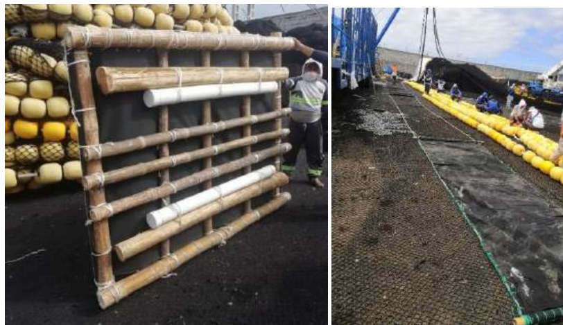
Figure 8 – Sails-type dFAD characteristic of the Eastern Pacific with a bamboo frame raft and extra PVC flotation (left) and a three-sail tail in the net yard of the port of Manta (Ecuador) (right).
