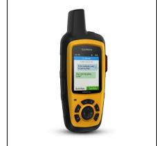
The device is not completely waterproof, but is water-resistant for 30 minutes up to 1 meter deep.
