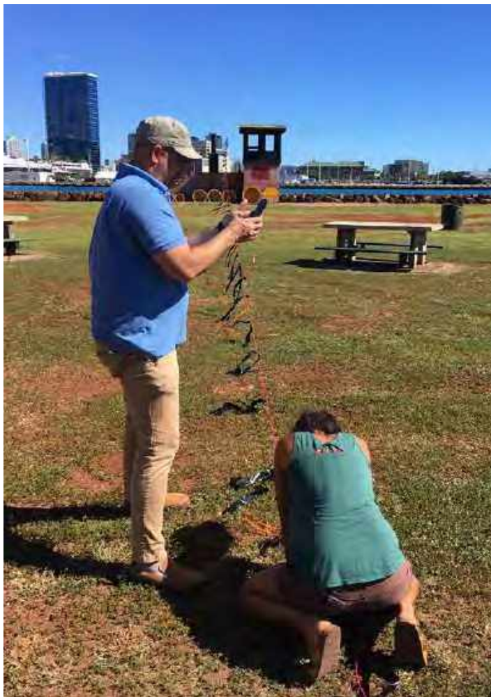
Colby Brady and Hollyann Naholowaa conducting tori line land trials to determine the necessary drag for each aerial section design under consideration. Credit: NOAA Fisheries/ Sarah Ellgen
