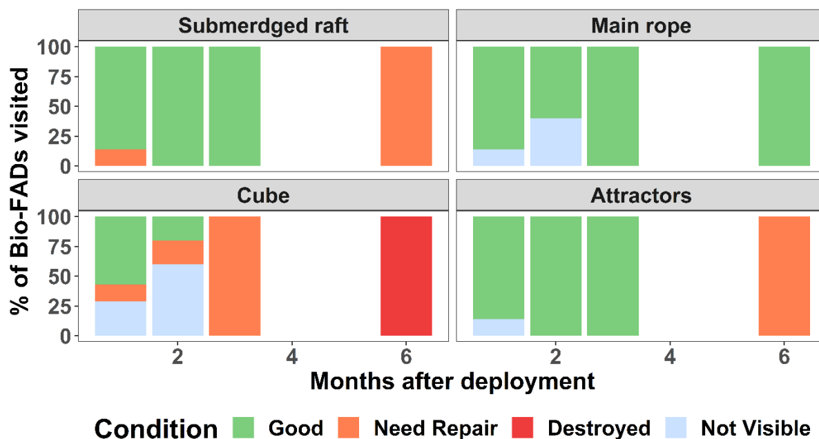
Figure 8. State of the different components of the 12 jelly-FADs with time at sea
