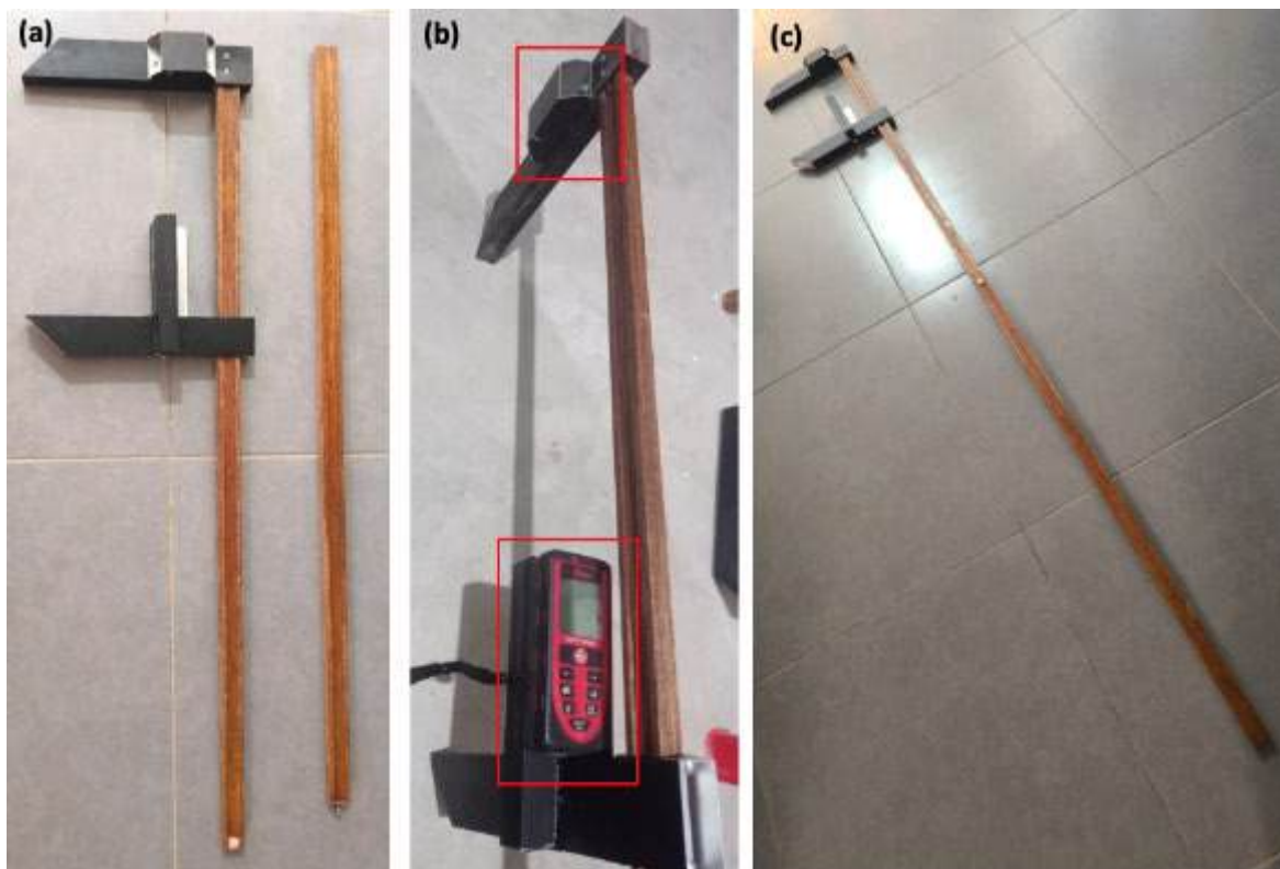
Figure 14. (a) Two-meter detachable ichthyometer adapted to a laser distance meter for taking morphometric measurements of elasmobranch species in Peru; (b) The red rectangles indicate the receiver and holder where the laser signal is received and where the laser is placed, respectively; (c) Ichthyometer at its full length of 200 cm.
