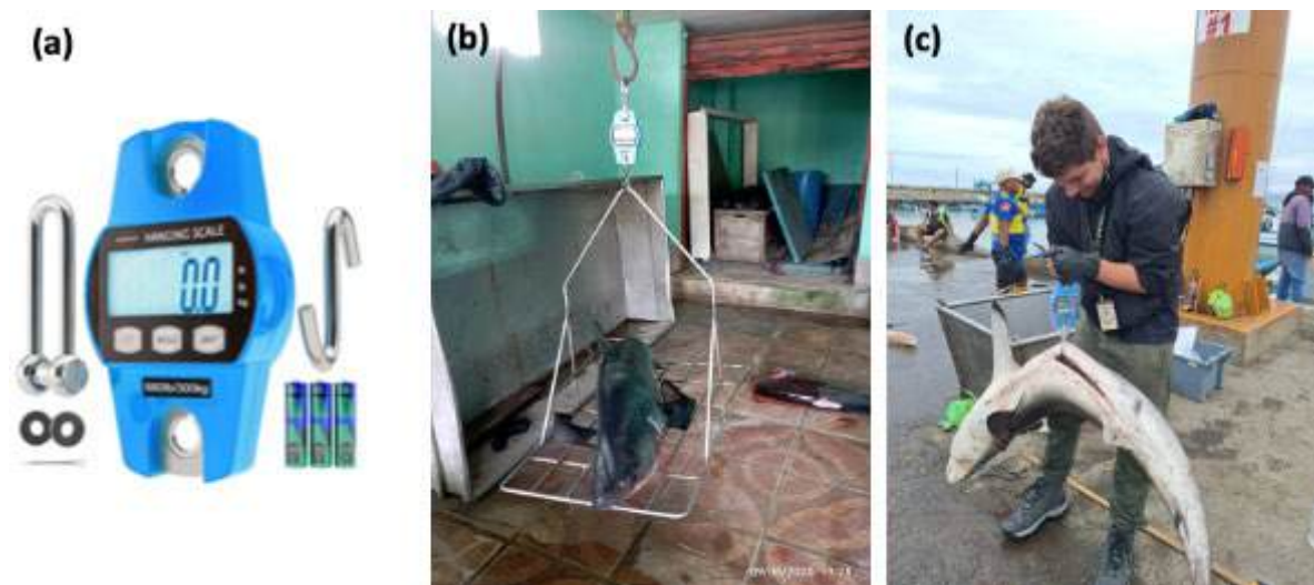
Figure 19. (a) 300-kg hanging scale for weighing larger individuals; (b) weighing a juvenile individual using a metal support; (c) manual weighing of a sub-adult individual without a support base at landing sites in Ecuador.
