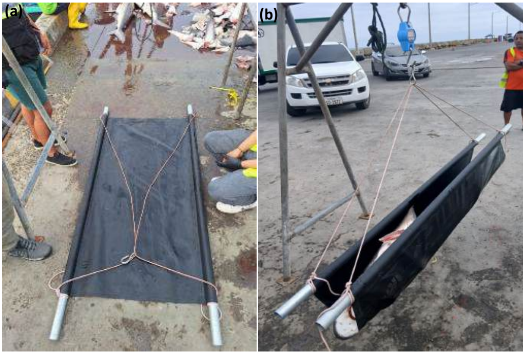
Figure 20. Use of a reinforced canvas stretcher for weighing juvenile and adult sharks at landing sites of Ecuador's longline mother vessel fleet; (a) Stretcher laid out on the ground prior to use; (b) Specimen being weighed using a hanging scale, with the stretcher as a support to distribute the weight and prevent damage.
