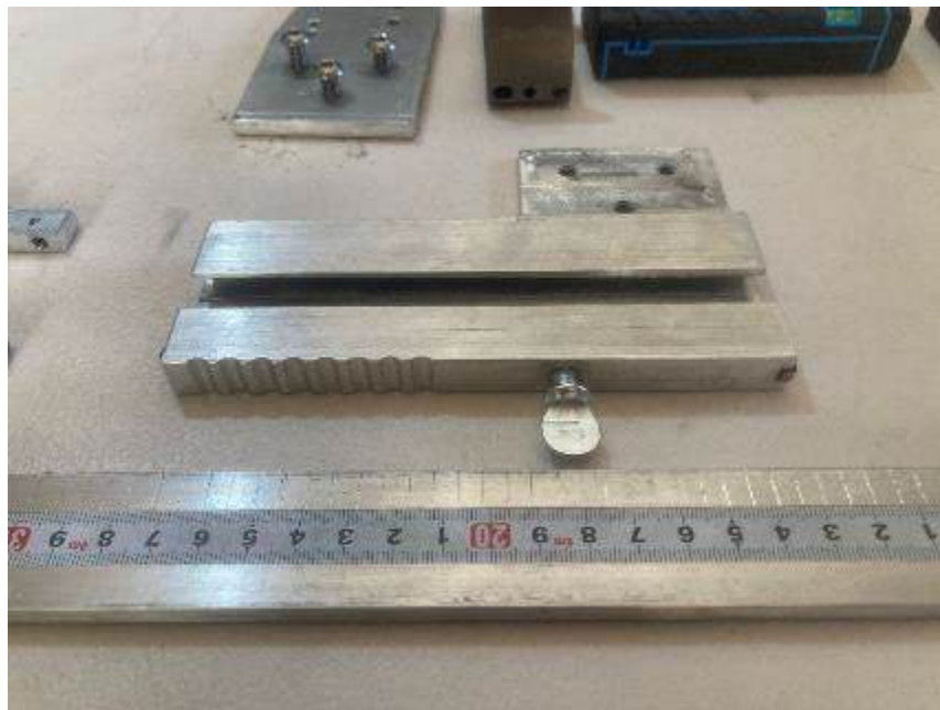
Figure 18. Saltwater-resistant measuring tape and grooves on the handle of the movable arm ensure a good grip during use in extremely wet conditions.
