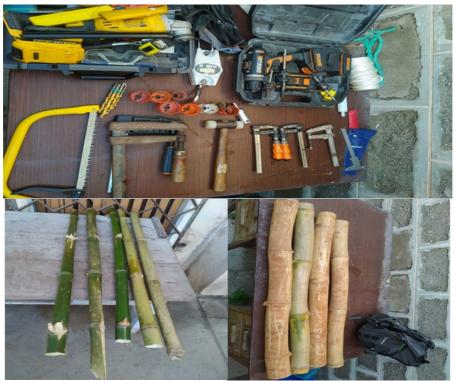
Figure 1. Tools and bamboo canes needed to build the biodegradable FAD.
