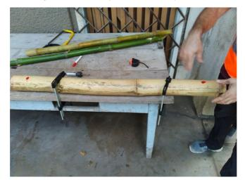
1. Clamp big bamboo canes (100mm diameter) onto work bench
