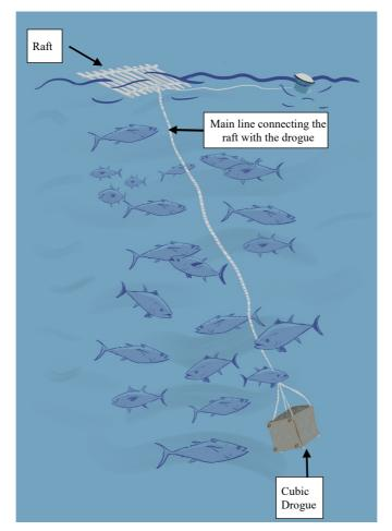
Figure 5. Conceptual drawing of the new DFAD design
