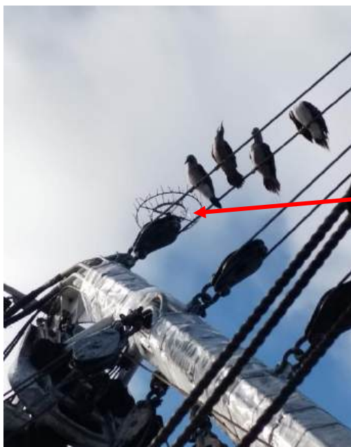
FIGURE 1. Image depicts an example of a protective device (red arrow) built by fishers on a purse seine vessel to prevent seabirds, taking refuge on the vessel, from getting caught and injured in the working lines.
