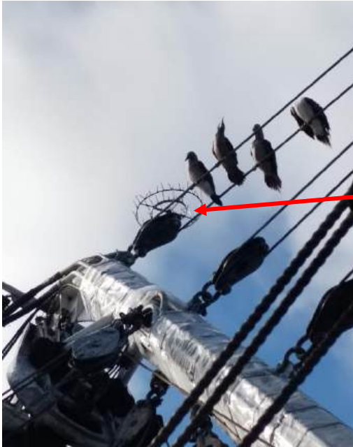
FIGURE 1. Image depicts an example of a metal cage protective device (red arrow) built by fishers on a purse seine vessel to prevent seabirds, taking refuge on the vessel, from getting caught and injured on one of the blocks in the working lines.
