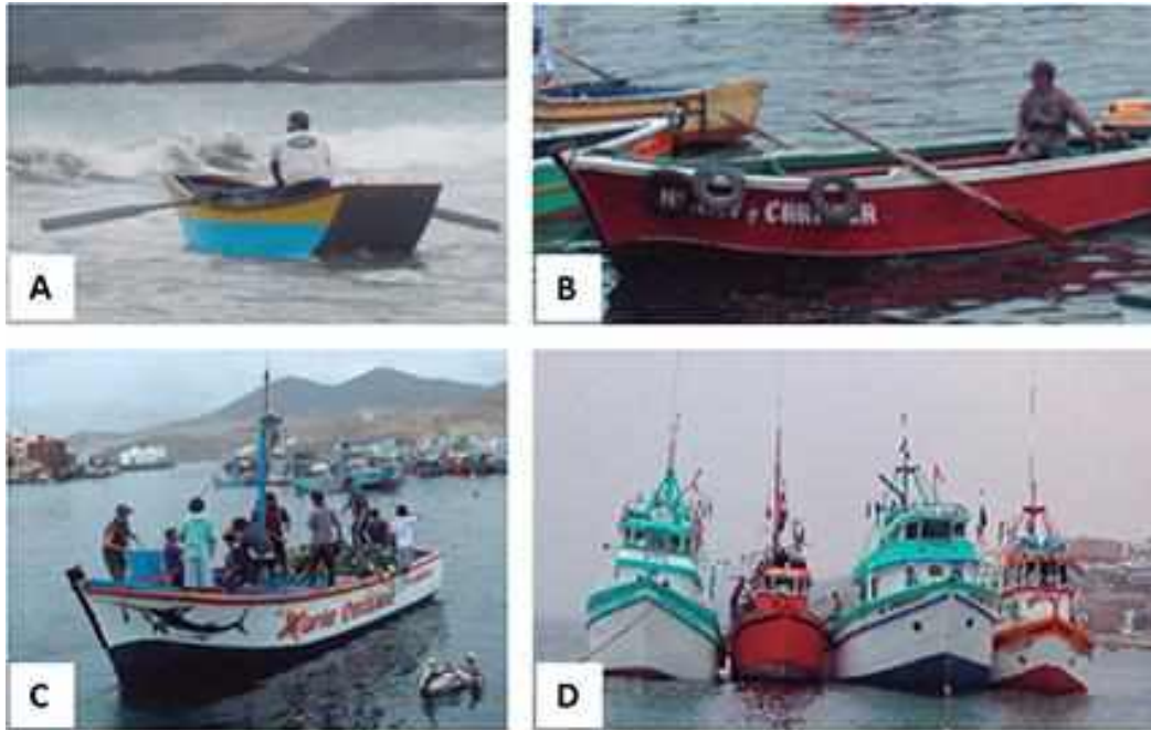
Figure 3. Classification of artisanal fishing vessels in Peru. The figure shows vessel types: A) zapato ; B) chalana , from Castillo et al. (2018); C) bote ; D) lancha , from Guevara-Carrasco and Bertrand (2017).
