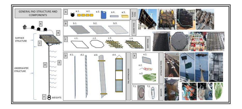
FIGURE 1. Designs of general dFAD structure and components including the materials found in their construction.
