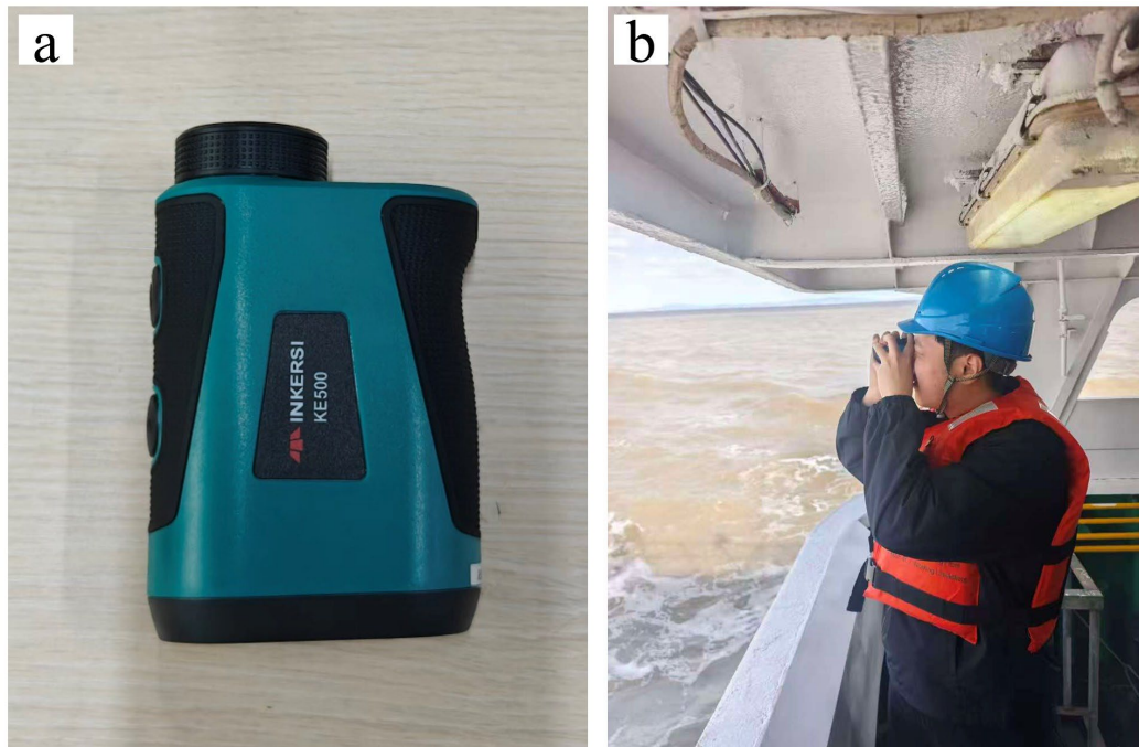
Figure 4 Schematic diagram of the aerial extent measurement equipment and field measurement procedure for the tori line (a: the INKERSI KE500 visual laser rangefinder; b: researchers measuring the aerial extent in the field)
