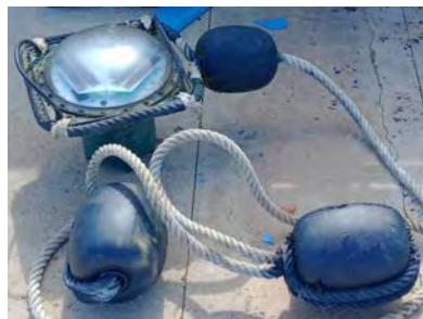
Plastic buoys (left) or purse seine corks painted blue with satellite/echosounder buoy (right)
