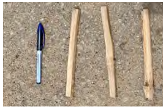
Wooden or bamboo pins to use as nails (with a pen to show scale)
