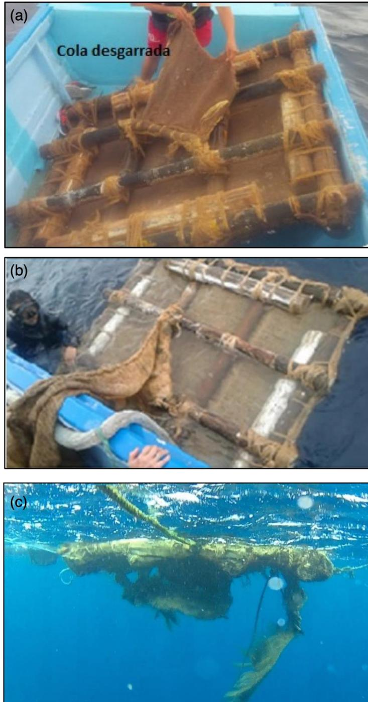
Figure 1: Biodegradation level of Eco-FADs constructed using jute (a), cabuya (b) and abaca (c) fibers
