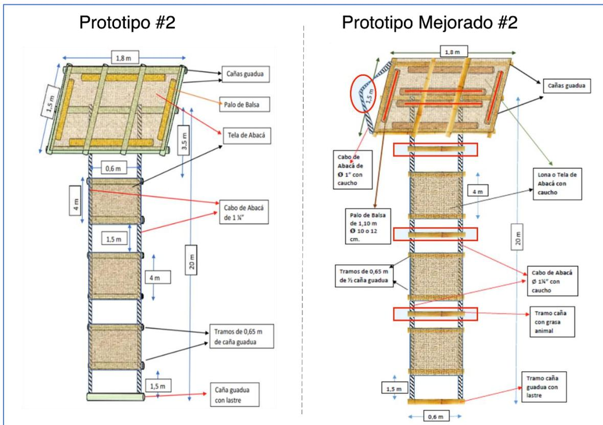
Figure 2: Design of Eco-FADs used in the framework of the CIAT project (left) and during the functional implementation period by the TUNACONS Foundation member companies (right)
