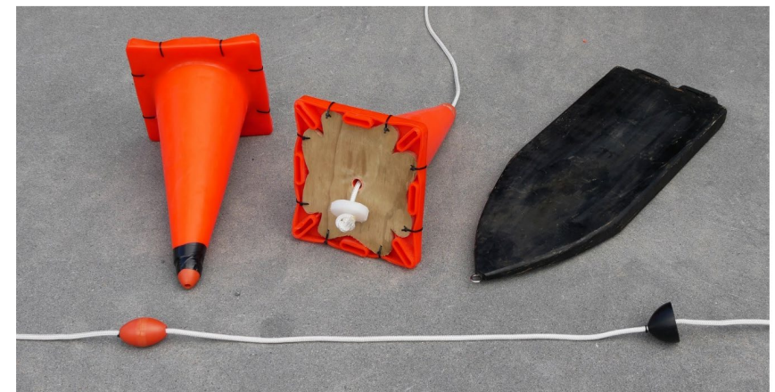
Figure 4: Drag section components for demersal longliners.
