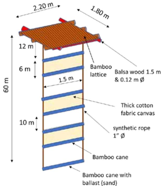
**FIGURE 19** Additions and modifications to improve durability of Prototype 3. Note that synthetic rope will only be used in the last batch of deployments (still pending). Deployments of 3<sup>rd</sup> quarter of 2021 consisted of NEDs with a biodegradable cotton-based rope that was successfully used and implemented in other ocean regions by some vessels of the same fleet.
