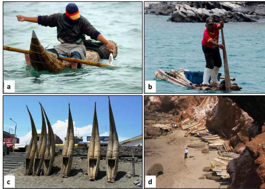
Figure 7. Traditional ancestral vessels used in Peru; a) caballito de totora (reed boat) and b) balsilla (raft), with their respective beaching methods (c and d).
