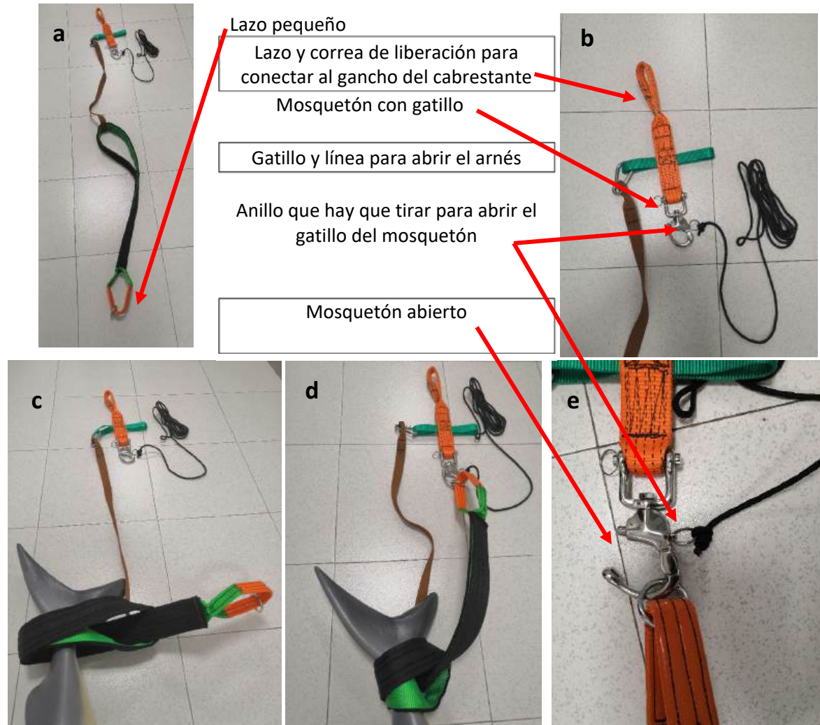
FIGURE 8. Shark harness (a) and configuration. In image (b) the loop that goes on the winch is shown zoomed in (orange strap) with the release trigger carabiner and the line attached to the release trigger for releasing the harness and the shark. In image (c) the small loop is passed through the large loop around the caudal peduncle of a shark. Image (d) shows the final set up with the ring on the small loop attached to the carabiner. Image (e) shows the strap with carabiner to attach the harness belt and rope tied to the trigger release ring which opens after pulling the rope sideways.
