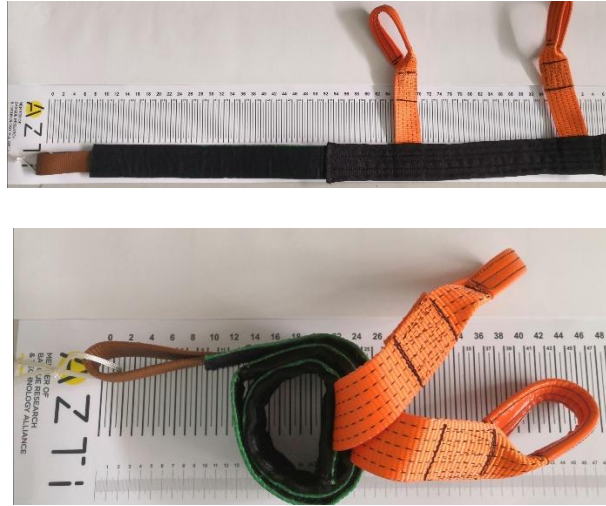
Figure 3. Small shark velcro extended (above) and closed (below).
