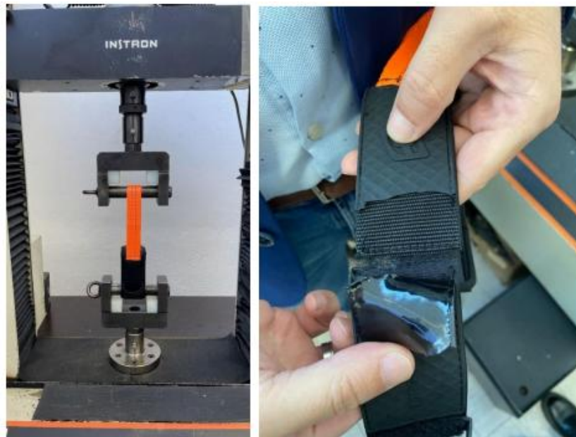
Figure 2. Adapted big wave surf leashes breaking during laboratory tests.
