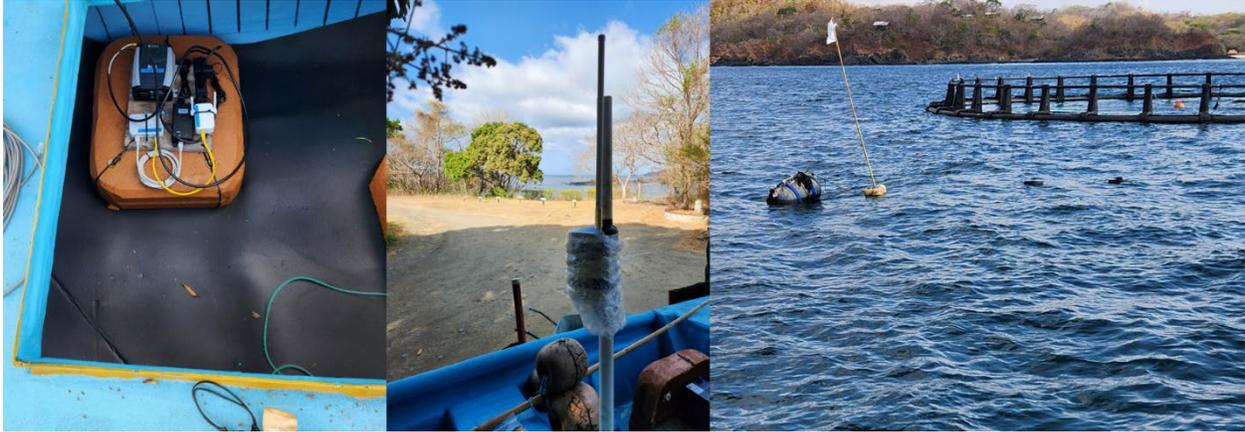
**FIGURE 3.** Equipment setup for the trials made in the Achotines lab, with the electrical and internet set up (left panel), hub (i.e., receiver) with the antenna (central panel) and the sensors (i.e., trackers, transmitters) on the satellite buoys (right panel).
