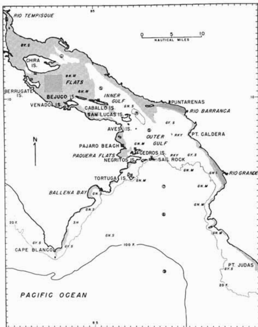
FIGURE 1. Map of the Gulf of Nicoya showing: depth contours in fathoms (shaded gray = less than 5 fathoms, dotted line = 20 fathoms, solid line = 100 fathoms); bottom types (GY.S = gray sand, GN.S = green sand, GN.M = green mud, RKY = rocky, SH = shell); seven hydrographic stations (station numbers circled); and principal areas fished according to gear used (trawling areas are striped and beach seine areas are cross-hatched).
