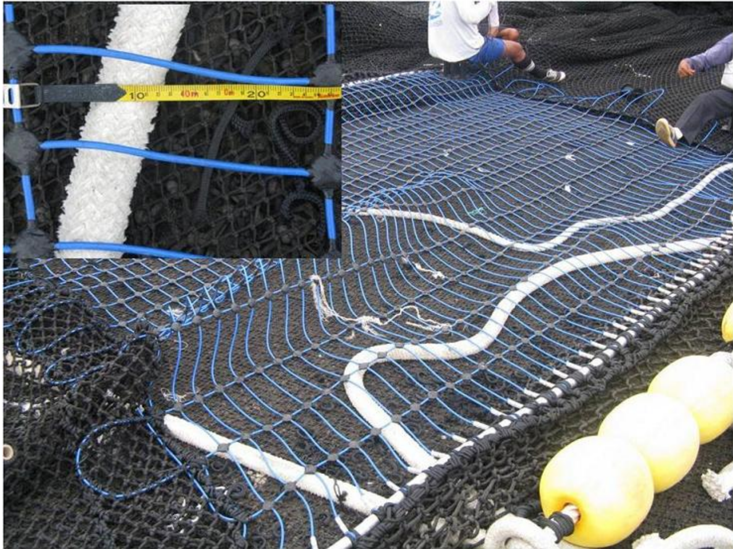
FIGURE 66 Arrue's sorting grid. Details of construction
