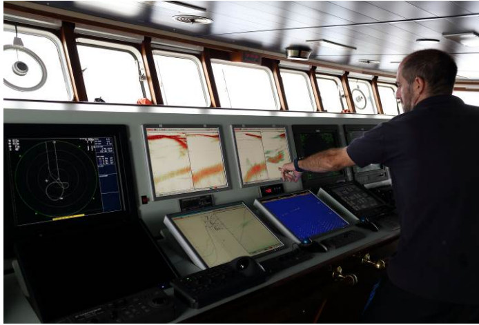
Fig.1 A captain using the information from the echo-sounders in the bridge
