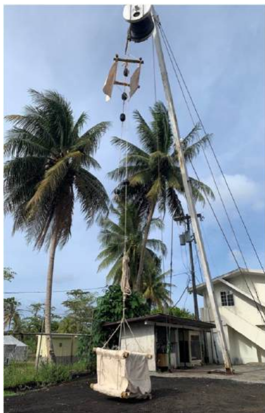
Figure 11. Jelly-FAD design with a cubic drogue. Photo: G. Moreno
