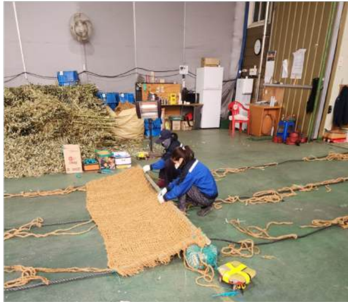
Figure 8. Bio-FAD used by Korean fleets, curtain-type dFAD made of bamboo, cotton rope, coir rope, and coir canvas, with chain as weight.
