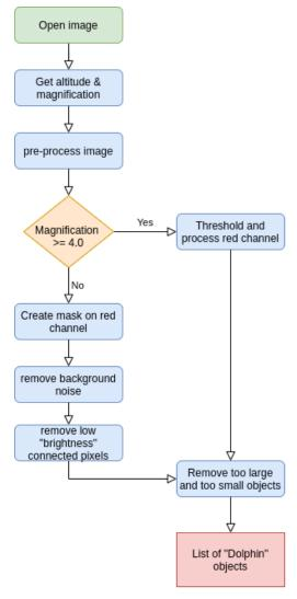
**FIGURE 1.** Overview of computer vision algorithm for the generation of dolphin objects for labelling by a human expert.
