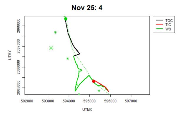
**FIGURE 49.** Example path of a calibration flight showing different modes with TOC: outbound transit (searching for school), WS: with school, and TIC: inbound transit (returning to the ship). Green and red dots indicate the locations of the drone during launch and landing, respectively. Green stars indicate the location of the initial sighting (big star) and resights (small stars). Date and flight number are given in the title. Units for UTM coordinates are meters.
