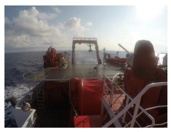
**FIGURE 5.** Platform for launching and landing drones on the back deck of the R/V Dr Jorge Carranza Fraser with a Seahawk S drone operated by pilots from Gtt NetCorp ready for take-off.
