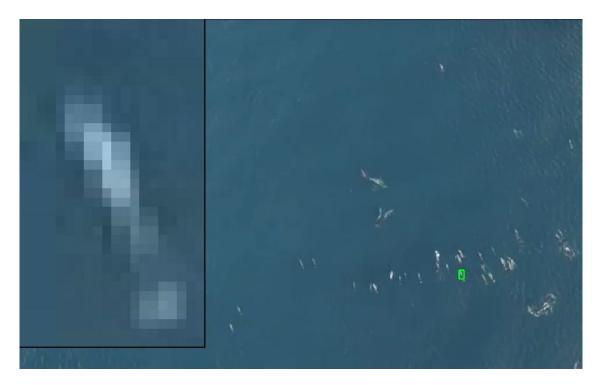
**FIGURE 9.** Example of the quality of the data demonstrating the poor pixel resolution. The enlarged section on the left shows the dolphin enclosed in the green box within the large frame. Without context of the large frame (or the video, not shown here), the object in the enlarged section is almost impossible for a human observer to identify accurately as a dolphin and it is entirely impossible to identify its species.
