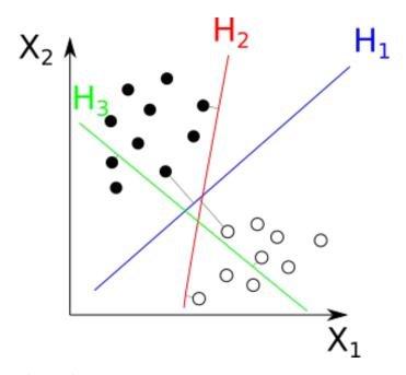
**FIGURE 20.** Example of classification using SVM including three hyperplanes, H1, H2, and H3, that could be used to define the two classes of points (black and white). H3 does not separate the classes. H2 does separate the classes but with only a small margin. H1 separates the classes with the optimal margin.
