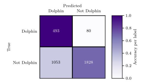
**FIGURE 21.** The confusion matrix for the motion model run on the validation data, with TP (493) and TN (1,828) on the diagonal, and FP (1,053) and FN (80) on the off-diagonal.
