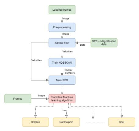
**FIGURE 16.** Overview of the motion analysis model. Green boxes indicate input data, blue boxes relate to training, the red box indicates the final predictive model, and the yellow boxes are the output labels.
