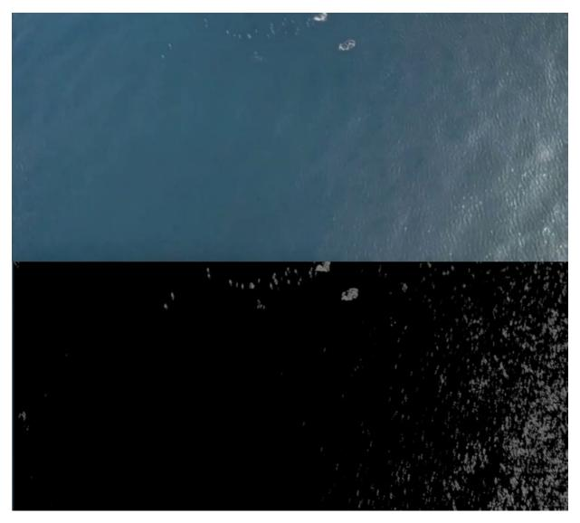
**FIGURE 18.** Example of the pre-processing of one still frame before it was fed into the optical flow algorithm. The bottom image shows the results of background subtraction and thresholding applied to the top image.
