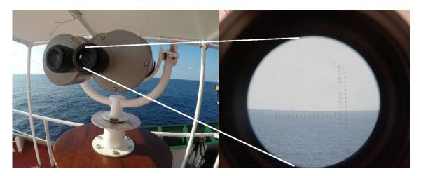
**FIGURE 4.** Bigeye binoculars (25 x 150 powered): the angle ring and pointer as well as the reticle scale in the right ocular allowed determination of the angle and radial distance of the detected dolphin school in relation to the ship.
