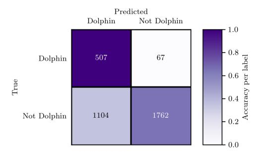
**FIGURE 15.** Confusion matrix for Densenet CNN model run on the validation data. The TP (507) and TN (1,762) are the diagonal entries. The off diagonals are the FP (1,104) and FN (67). The Densenet model was biased towards classifying the images it received as input as *dolphins*.
