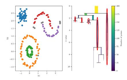
**FIGURE 19**. Example of the HDBSCAN algorithm clustering data. The left image shows the data where each cluster was given a different colour based on which cluster it belonged to. The right image shows the dendrogram for the data on the left. The five clusters were taken from parts of the dendrogram with the largest leaves. The largest leaves in this example are circled in red. Here, lambda ( $\lambda$ ) is the local threshold value.
