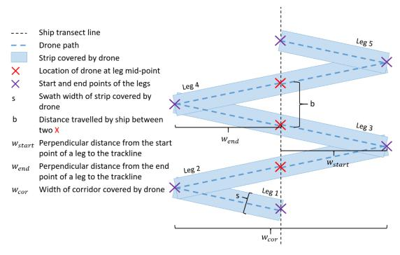
**FIGURE 38.** Diagram of theoretical drone flight path consisting of five zigzag legs in relation to the ship transect line. Not shown are the outbound and inbound transits from and to the ship.
