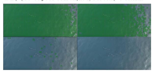
**FIGURE 42.** Example output from the image model. The bottom right panel shows the input image before patches were created. Top left (threshold of 50%), top right (threshold of 65%) and bottom left (threshold of 90%) panels summarize the output from the model using different likelihood thresholds. The green boxes indicated the patches that were labelled by the model as *dolphins*.
