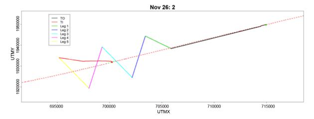
**FIGURE 36.** Example zigzag flight showing the different effort modes of the drone. TO: outbound transit, TI: inbound transit and on effort in search mode during 5 zigzag legs. Red dashed line indicates the ship track while flying bridge was on effort in passing mode. Green and red dots indicate the location of the drone during take-off and landing, respectively. Date and flight number given in the title. Units for UTM coordinates are meters.
