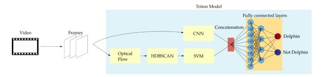
**FIGURE 22.** Diagram showing the Triton model, including the data pipeline. The video was split up into individual frames and fed into the model. The frames took two distinct paths through the model: the motion data analysis is shown in the lower path and the image analysis is shown in the upper path. These paths were joined at the concatenation stage, and then fed through the fully connected layers for classification.
