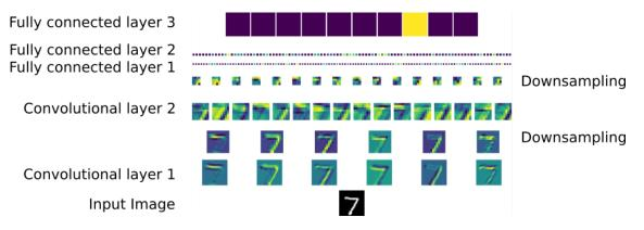
**FIGURE 14.** Example of a CNN classifying a hand drawn number. The image of the number is fed into the CNN (bottom layer). The convolution layers generate the feature maps which are then shrunk by the max pooling layers before the features are fed into the fully connected layers (neural network). The fully connected layers then classify the image correctly (result layer, not shown).
