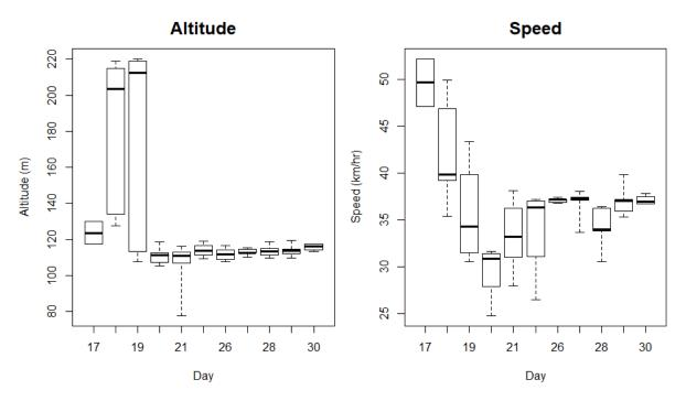
**FIGURE 37.** Drone altitude and speed distributions, by day, for the 300 zigzag legs. Horizontal bars represent medians, boxes the interquartile ranges and whiskers reach to the extreme values.
